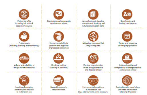
Figure 2.17: Examples of factors to consider during planning and delivery of a beneficial use project.
